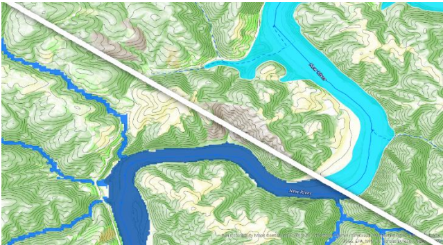
Fathom fluvial and pluvial flood areas (left) include smaller drainage areas not covered by available FEMA flood hazard maps (right).
