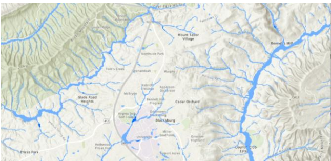
Maps depicting the 1% AEP (1 in 100 year) recurrence interval flood event in the Blacksburg area. Top: FEMA’s National Flood Hazard Layer. Bottom: the 2020 Fathom flood layer.
