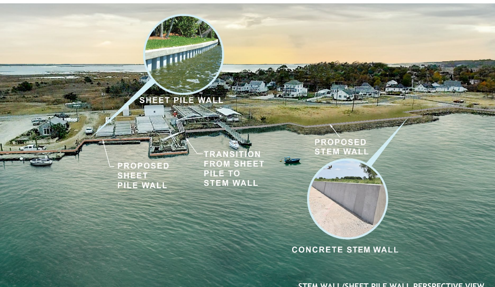
STEM WALL/SHEET PILE WALL PERSPECTIVE VIEW
